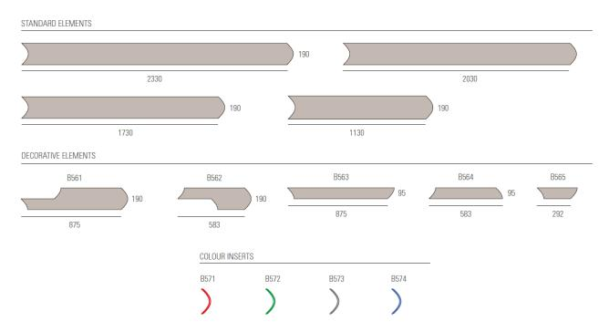
The modules called "decorative elements" are staggered in width by half a board compared to the "base" modules. Since all modules have a convex surface, where the centre line of a module (maximum thickness of the convex profile) meets with the side of the other element halved in width (minimum thickness of the convex profile), it creates a difference in level which is a characteristic of the material and it is not due to any kind of defect or deformation.
